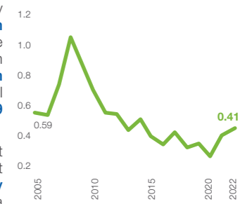
SF LEAKAGE AS A PERCENTAGE OF TOTAL GAS INSTALLED (%)
